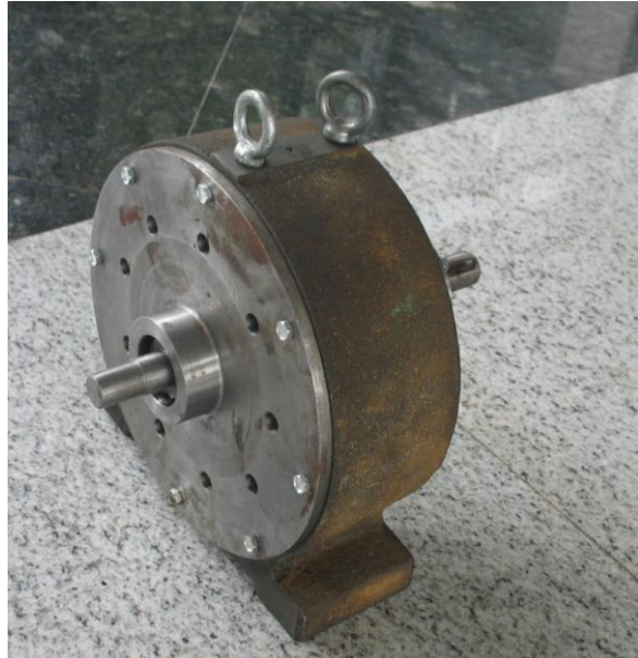
Fig.2. The world first sample of the swinging planetary drive of bevel gears
